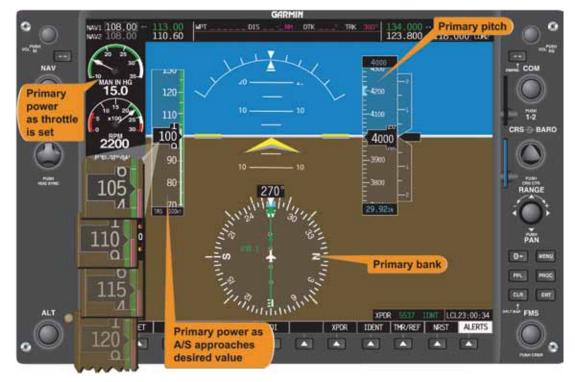
Figure 5-58. Straight-and-Level Flight (Airspeed Decreasing).
