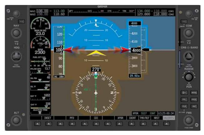
Figure 5-62. The pilot has fixated on pitch and altitude, leaving bank indications unattended. Note the trend line to the left.
