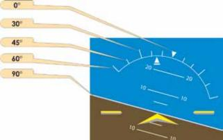
Figure 5-53. Attitude Indicator Showing a 15° left bank.
