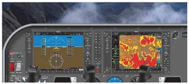
Figure 5-48. Pitch Attitude Decreasing and Airspeed Increasing—Indicates Need to Increase Pitch.
