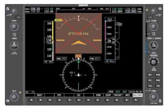
Figure 5-73. AHRS Unit Failed.
