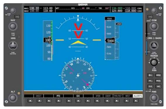
Figure 5-69. Unusual Attitude Recovery Protection. Note the brown horizon line is visible at the bottom.
