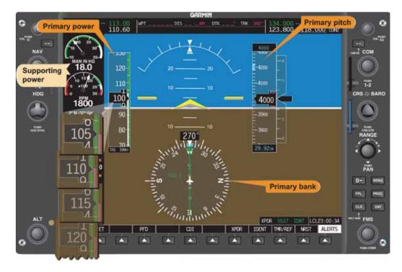
Figure 5-59. Straight-and-Level Flight (Reduced Airspeed Stabilized).
