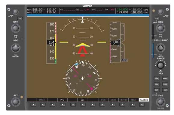
Figure 5-70. Horizon line starts moving upward at 27°. Note that the blue sky remains visible at 17° nose-down.
