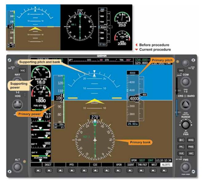
Figure 5-64. Constant-Airspeed Climb From Established Airspeed.
