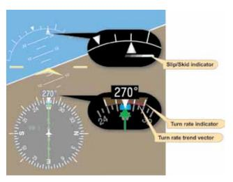
Figure 5-54. Slip/Skid and Turn Rate Indicator.
