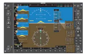
Figure 5-50. Pitch Indications for Various Attitudes (1° through 5°).
