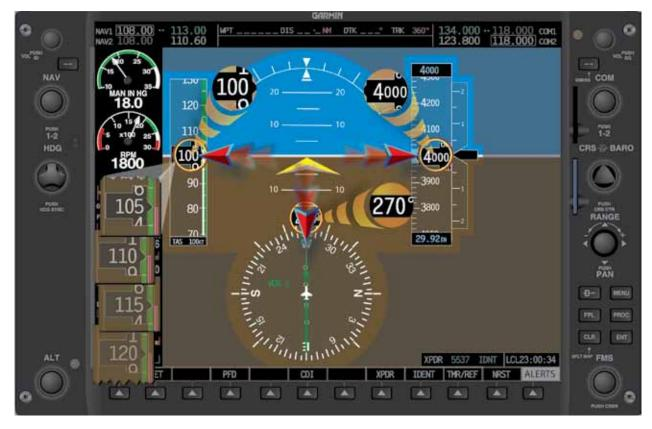
Figure 5-61. Insufficient cross-check. The problem is power and not nose-high. In this case, the pilot decreased pitch inappropriately.
