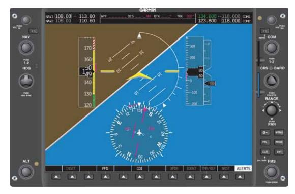
Figure 5-71. Aircraft Rolled Past 60°.
