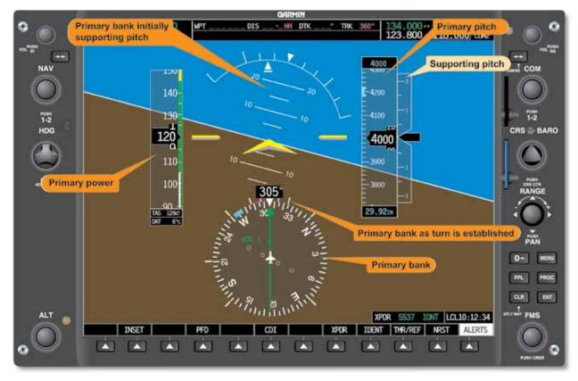
Figure 5-67. Standard Rate Turn—Constant Airspeed.
