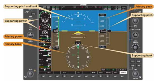
Figure 5-57. Straight-and-Level Flight (Normal Cruising Speed).
