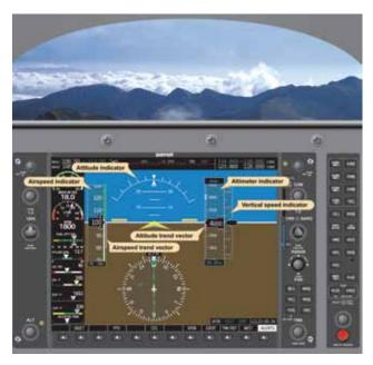
**Figure 5-47.** *Pitch Attitude and Airspeed in Level Flight, Slow Cruise Speed.*
