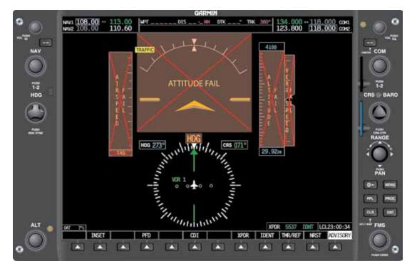
Figure 5-74. AHRS ADC Failure.
